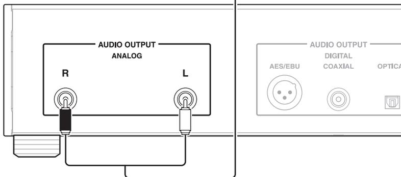
This is an example of analog connection using the preamplifier P-3000R.
