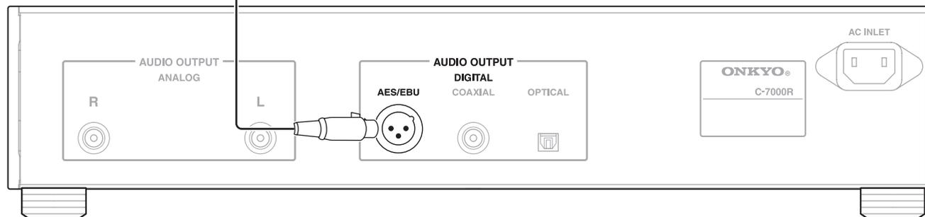
This is an example of AES/EBU connection using the preamplifier P-3000R.
