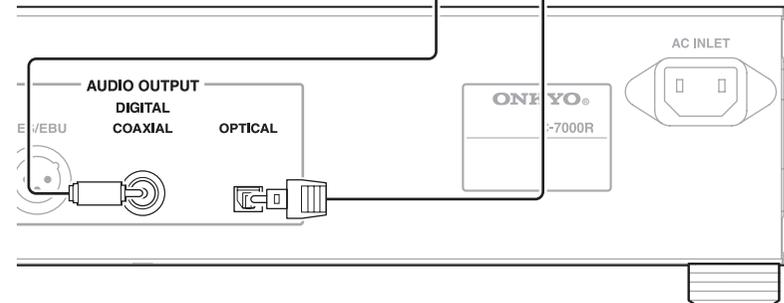
This is an example of digital connection using the preamp P-3000R.
